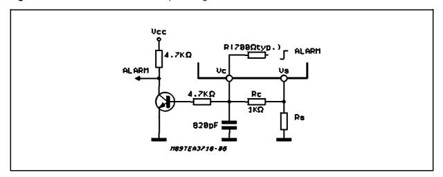
Figure D: CommonDetection for Several Multiwatt Package
