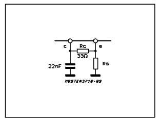
**Notes:** 1. Resistance values given here are for the V<sub>ch</sub> threshold. They should be adjusted using other comparators threshold or other V<sub>ref</sub> value.
