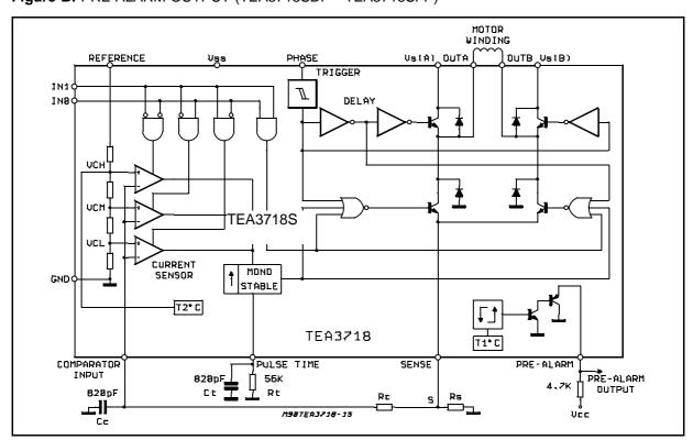
**ALARM OUTPUTS** (TEA3718SP - TEA3718DP) The alarm output becomes low when the junction temperature reaches  $T^{\circ}C$ .
