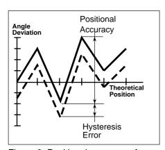
Figure 9. Positional accuracy of a stepper motor.
