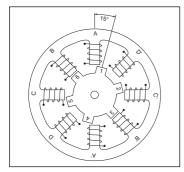
Figure 1. Cross-section of a variable-reluctance (VR) motor.
