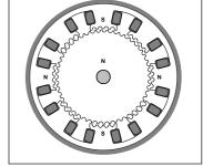
Figure 3. Cross-section of a hybrid stepper motor.
