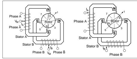
Figure 6. Unipolar and bipolar wound stepper motors.
