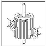
Figure 2. Principle of a PM or tin-can stepper motor.
