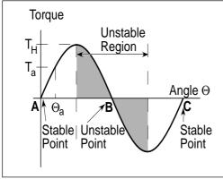
Figure 7. Torque vs. rotor angular position.
